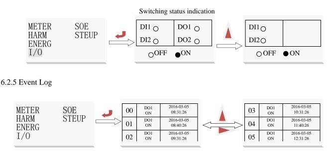
The instrument displays the action information of the switching inputs and outputs by pressing the Enter key after the event record is selected. As shown above, the 1st record indicates the 1st switch input at 8:31:26 on 5/3/16; the 5th record indicates the 1st switch input at 12:31:26 on 5/3/16. Press the up and down keys to view other records, and a total of 16 records are saved.
