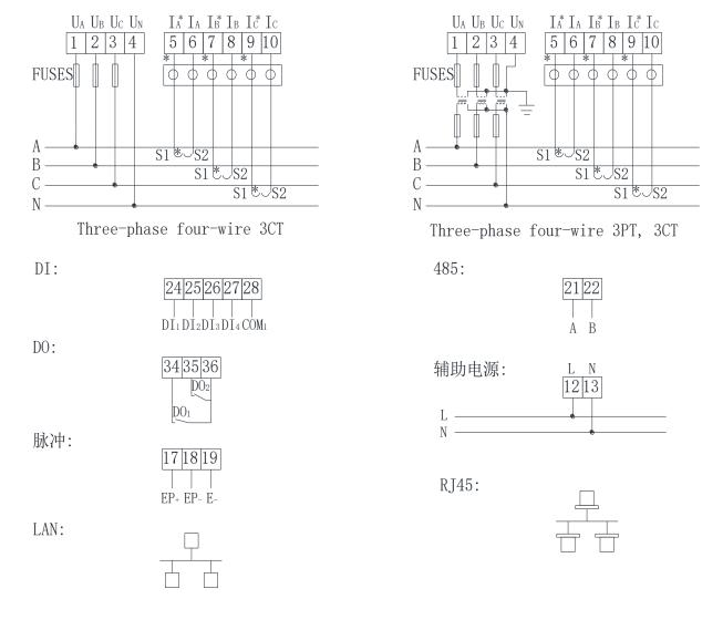
It is recommended to use 3A fuses in the wiring diagram
