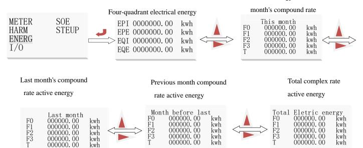
1. The four quadrants are forward active energy, reverse active energy, inductive reactive energy and capacitive reactive energy, generally speaking, the user reads the forward active energy EPI.
